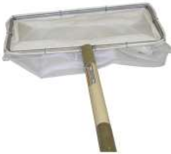
Figure 6.2 Standard kick net (500µm) used for collecting benthic macroinvertebrates.
